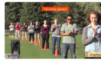
SPH3U - Keep in Time! Measuring the Speed of Sound Students use observe the progression of sound waves, watching marching band musicians clapping to the sound of a metronome.
