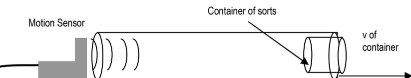
Now, while collecting position vs. time data, slowly draw the play-doh container out of the tube. When you get to the physical end of the tube, stop and hold a few seconds. Now slowly continue to draw the container out further.
