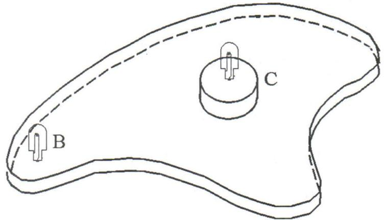
We first cover bulb B. We give the "amoeba" a push and watch it travel over the air table. Bulb C travels in straight lines, changing direction only when the "amoeba" bounces off the edges of the air-table.
