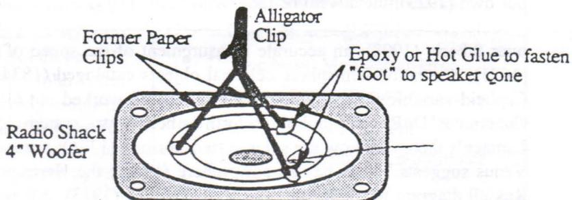
For longitudinal vibrations, use a light spring, and place the demonstration on an overhead projector (see diagram). I found the spring from my Pasco dynamics cart set worked very well. You can illustrate the characteristics of nodes, antinodes, and changing mode number with changing frequency. It is possible to use a hand stroboscope to slow the action down so that the motion of the coils at the nodes can be studied.
