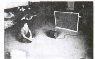
Fig. 1. The dark set is receiving electromagnetic waves from the white transmitting set directly and also by reflection from the window screen.
